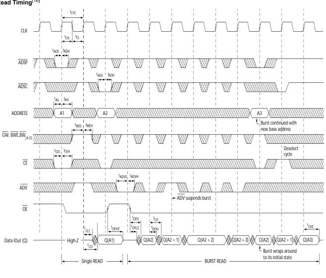
16. On this diagram, when  $\overline{CE}$  is LOW,  $\overline{CE}_1$  is LOW,  $\overline{CE}_2$  is HIGH and  $\overline{CE}_3$  is LOW. When  $\overline{CE}$  is HIGH,  $\overline{CE}_1$  is HIGH or  $\overline{CE}_2$  is LOW or  $\overline{CE}_3$  is HIGH.
